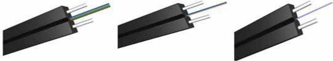
Optic unit is set in the center of the cable. On either side of it there are two strengthening constructions made of ultraviolet-resistant and fire-proof polymer material (LSZH - oxygen index higher than 33). Steel wire guide lines inside the polymer base allow preventing unallowable bending and coiling.
